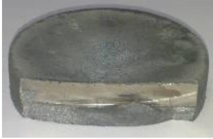
Fig. 1. Overview of RM semi-product based on NiAl produced by centrifugal SHS casting in optimal conditions
