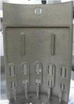
Fig. 4. Harvesting single segment produced by selective laser fusion of metal-powder composition CoCrMo.
